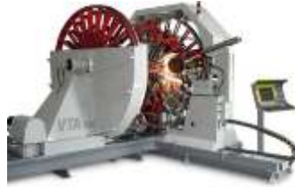
Fig: Welding Setup in rotating cage type assembly
